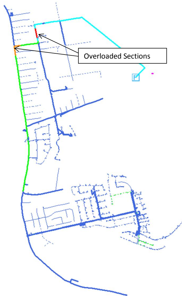
Figure 5.1. Overloaded sections on circuit CC7.
