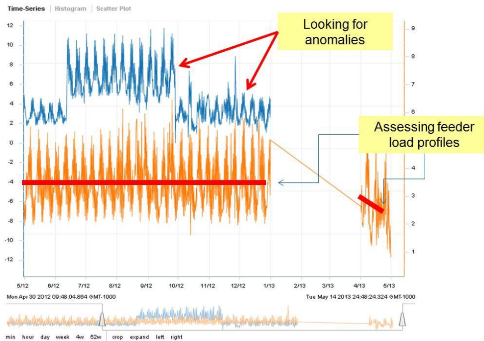
Figure 2.6. Example of load switching on the feeder where load was unusually high for a short period of time.
